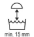
The symbol indicates that the distance from the underside of the light to the highest water mark must be a minimum of 15 mm.
