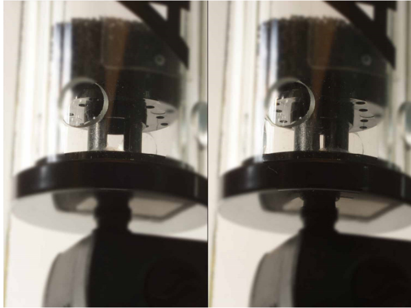
Picture 2: Regulating flow is done through changing the width of the gap inside the reactor, by turning the knob on top of the unit. The pump is connected at the bottom of the unit and can be adjusted as well.
