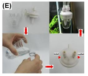
5.) Open the bubble counter & check valve, fill it up with water and then close it (Hand tighten). Make sure the check valve is connected in the right direction. Follow the triangle on the check valve to find the inlet and outlet connection. Push the hose all the way to the end of the fittings. Turn the fastening node clockwise and hand tighten to secure the tubes to prevent CO2 from bursting out. (E)
