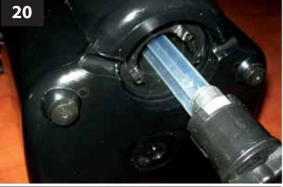
Tighten up to form a triangle of the socket and quartz glass
