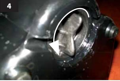
Remove the plug from the bottom of the filter container by unscrewing it
