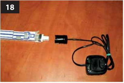
Install the light bulb in the UVC lamp socket
