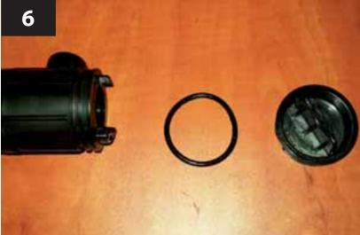
Take the gasket (oring) off the filter container plug and put it on the UVC lamp tube (regards the old version – in new models the lamp is already equipped with oring)
