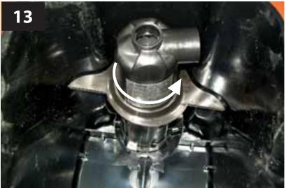
After installing UVC tube, move the flow cover towards the bottom of the container
